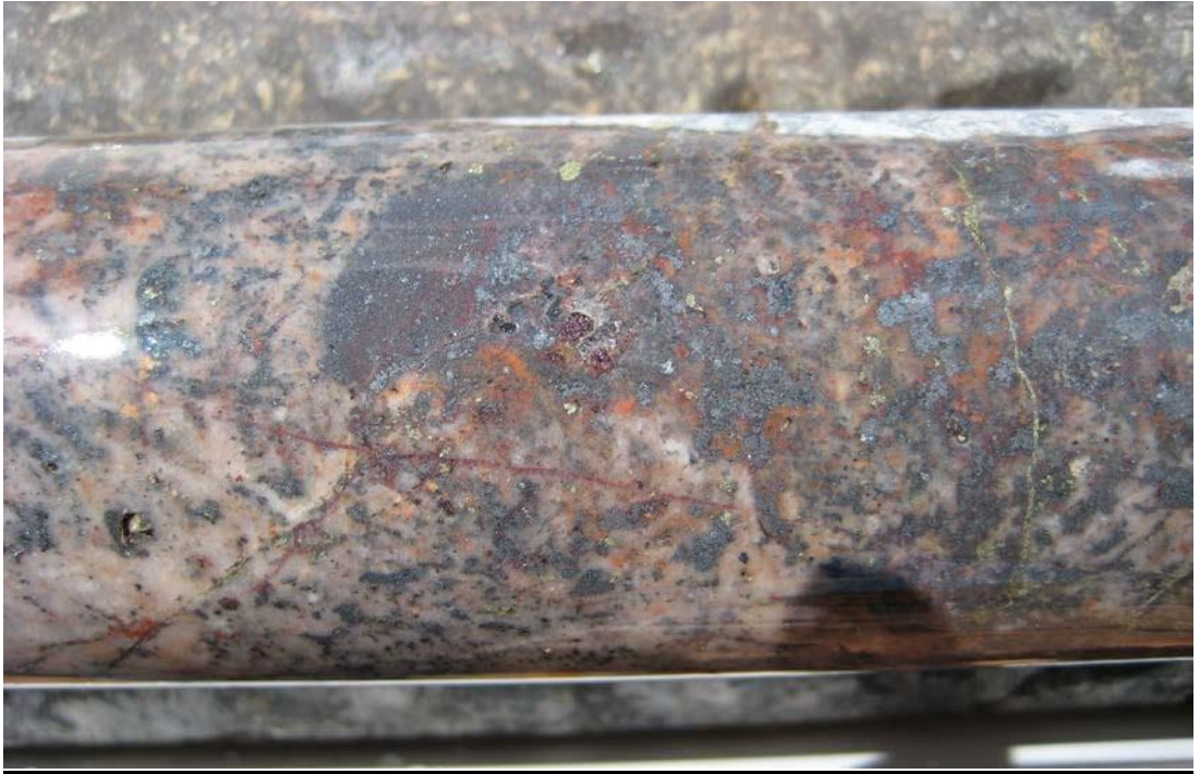
Figure 4: Close up photo of NQ size diamond drill core from 917m depth in VUD 8. Visible is disseminated bornite (purple coloured near centre of photo) chalcopyrite (a different copper iron sulphide mineral, yellow) with associated with hematite (grey and reddish) in a very highly silicified breccia host rock. Width of photo is about 15cm.
