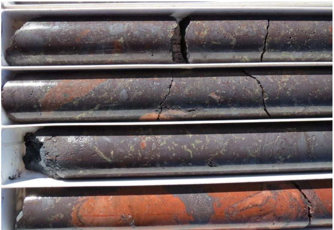
Figure 5: Detailed photo of mineralised hematite breccias within VUD 15. The grey/black mineral is hematite (iron oxide), the main, lighter (pale yellow) mineral is pyrite (iron sulphide) with chalcopyrite (copper-iron sulphide) and the red material at the base of the photo is a fragmented dyke.
