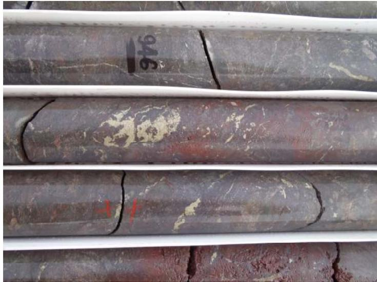
Figure 4d: VUD 12 946m, coarse chalcopyrite in hematite-rich breccia/massive hematite (NQ2 core)
