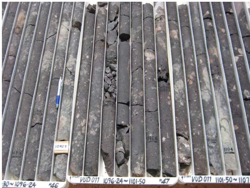
Figure 3a: VUD 11 1082-1106m, vuggy hematite-rich breccia (NQ 2 drill core)
