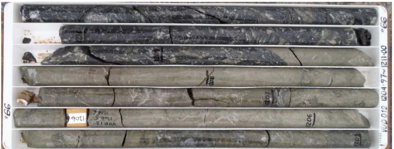
Figure 4e: VUD 12 1204.97-1211.00m, strong sericite-carbonate alteration (pale greenish, bottom rows) and chlorite carbonate-breccia (top rows) NQ2 core.
