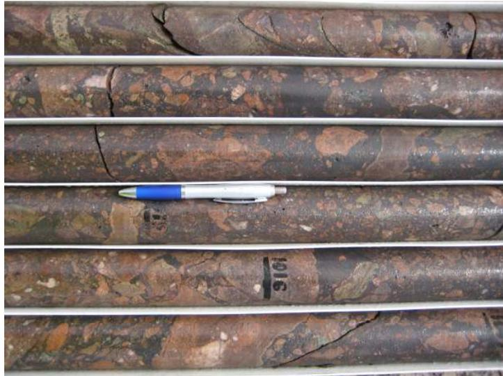
**Figure 3c: VUD 11 1015m, hematite (matrix) – rock fragment breccia (NQ2 core).**
