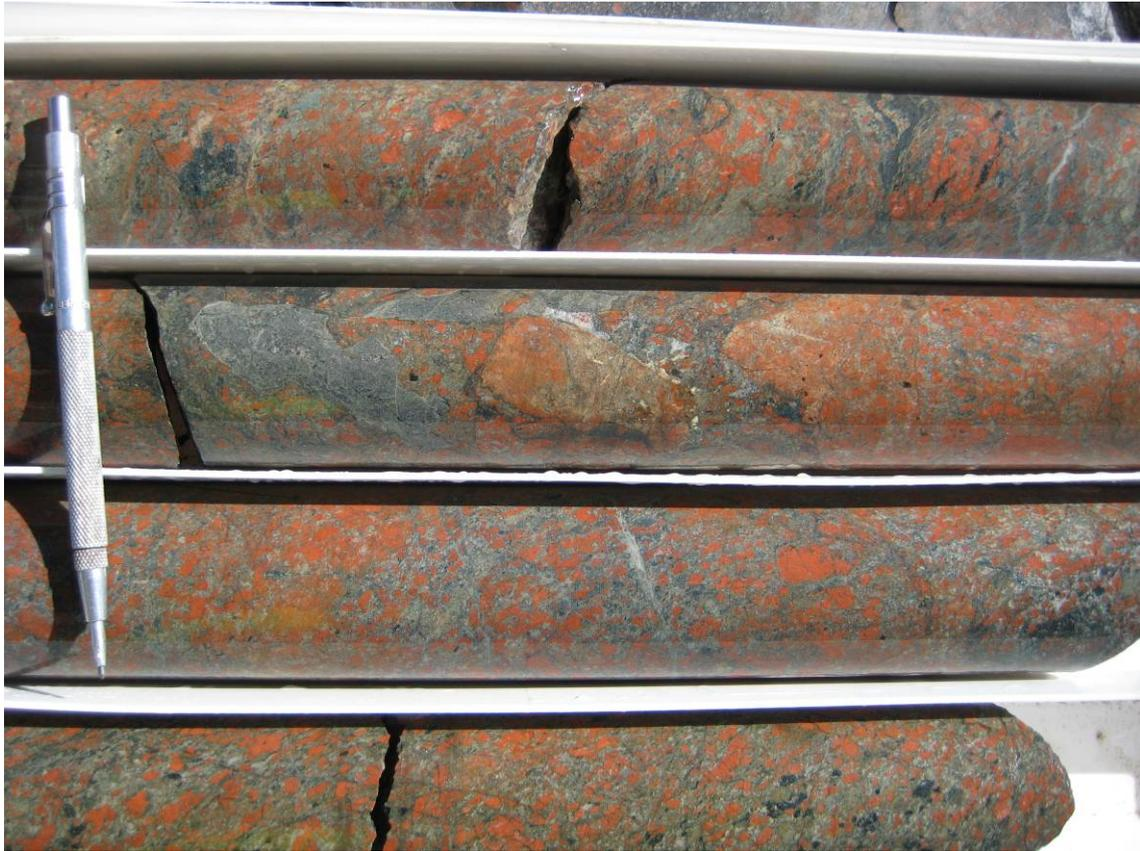
**Figure 2: Altered basement rocks in NQ size drill core from VUD 014 at about 980m depth. The red/orange mineral is feldspar, and grey/greenish minerals are sericite, carbonate and quartz.**
