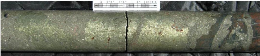
**Figure 3: VUD 3, massive pyrite/chalcopyrite (NQ drill core)**
