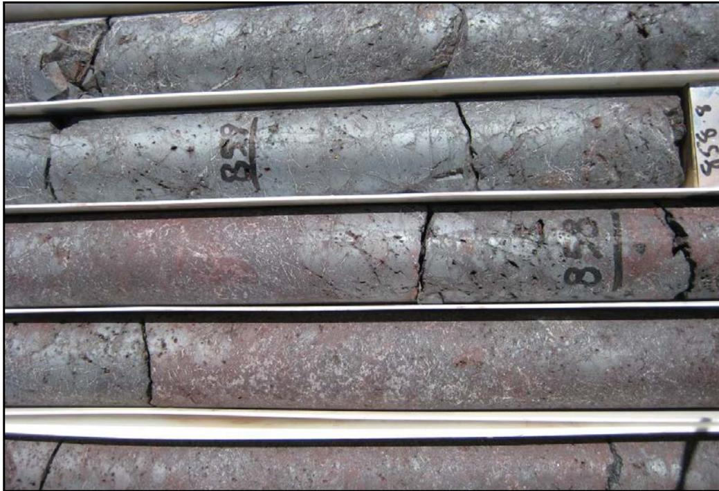
**Figure 2: Detailed photo of hematite breccias intersected in VUD 9 (NQ 2 drill core).**
