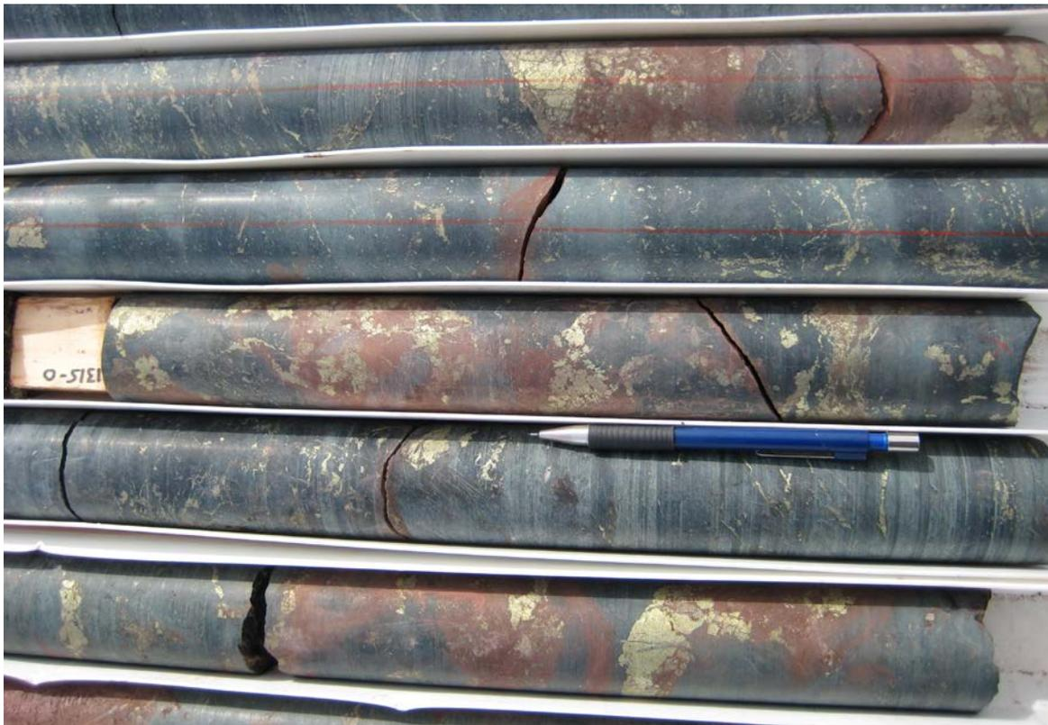
**Figure 4: Detailed photo showing chalcopyrite-pyrite mineralisation in a seven metre thick (down hole) intersection of probably remobilised IOCGU mineralisation within an intrusive dyke near the base of the VUD 15.**
