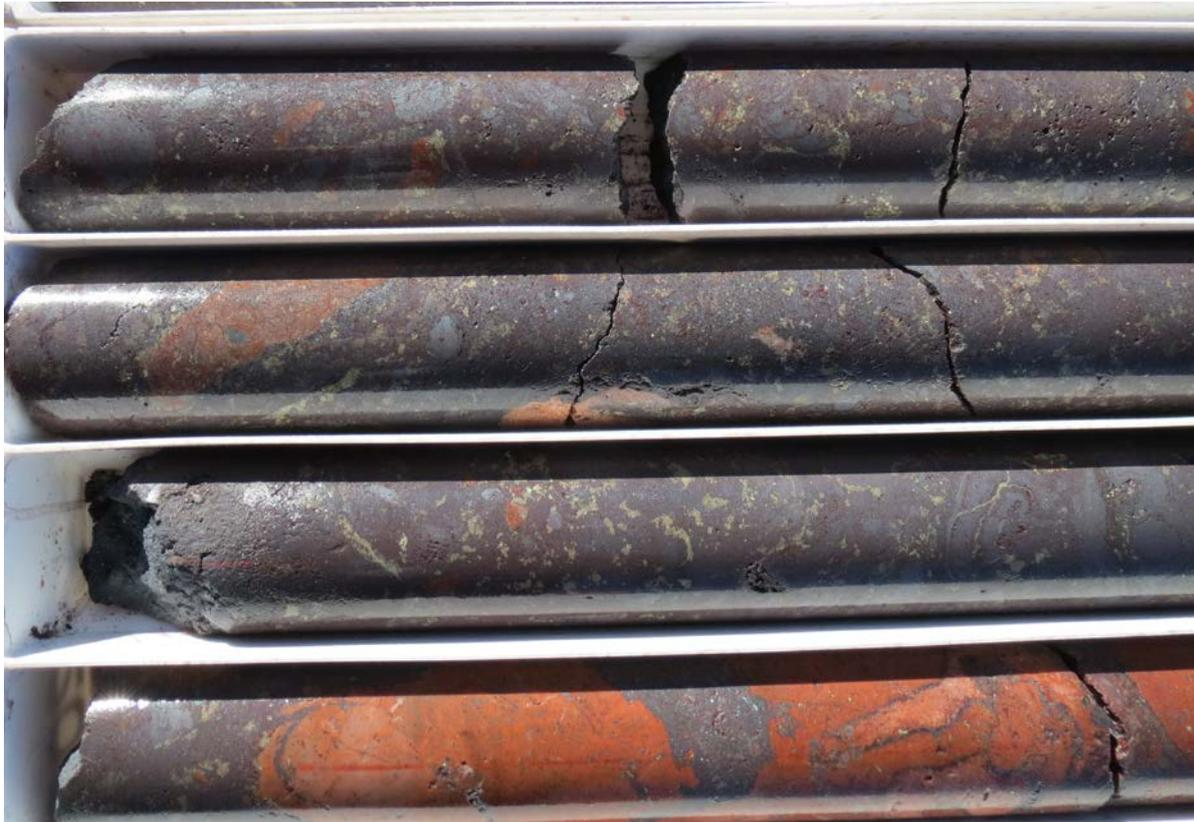
**Figure 3: Detailed photo of mineralised hematite breccias. The grey/black mineral is hematite (iron oxide), the main, lighter (pale yellow) mineral is pyrite (iron sulphide) with chalcopyrite (copper-iron sulphide) and the red material at the base of the photo is a fragmented dyke with bands of the red/orange mineral barite (barium sulphate, a common gangue in IOCGU deposits).**
