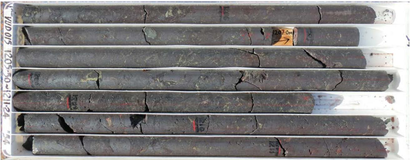
**Figure 2: NQ diamond drill core from VUD 15, showing pyrite-chalcopyrite mineralised hematite breccias. The grey/black mineral is hematite (iron oxide), and the main, lighter (pale yellow) mineral is pyrite (iron sulphide) with chalcopyrite (copper-iron sulphide).**
