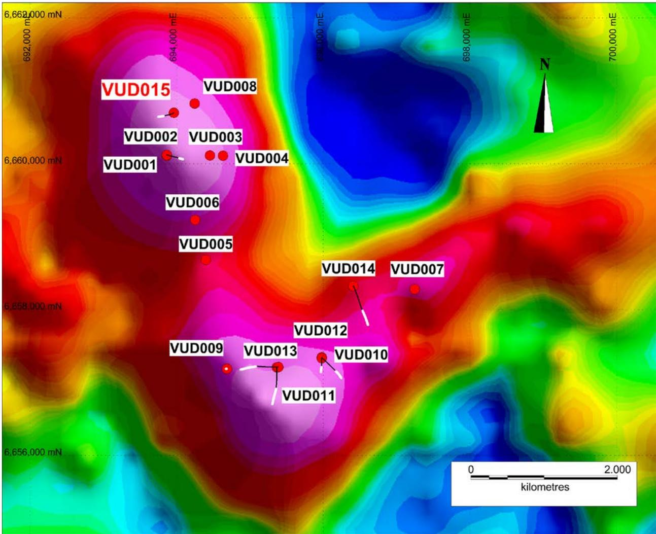
**Figure 1: Vulcan Project: residual gravity image showing all drill holes with recently completed VUD 15 labelled in red (GDA 94; MGA Zone 53). Surface projections of basement intersections in the inclined holes are shown in white. These projections show how relatively little of the Vulcan target has been tested.**
