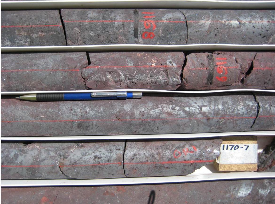
**Figure 2: VUD 16: Massive hematite breccia (NQ drill core).**
