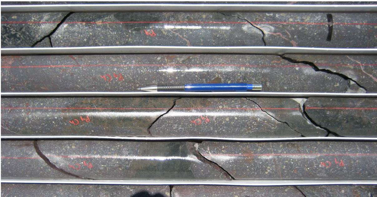
**Figure 5: VUD 17: Detailed Photograph of mineralised hematite-rich breccias. The grey mineral is hematite (iron oxide) and the fine grained lighter coloured minerals are the sulphides pyrite (iron sulphide) and chalcopyrite (copper iron sulphide), and carbonate minerals (NQ drill core).**
