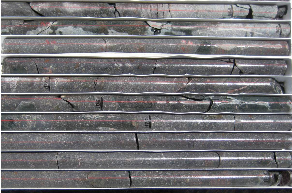
**Figure 4: VUD 17: Mineralised hematite-rich breccias. The grey mineral is hematite (iron oxide) and the fine grained lighter coloured minerals are the sulphides pyrite (iron sulphide) and chalcopyrite (copper iron sulphide), and carbonate minerals (NQ drill core).**
