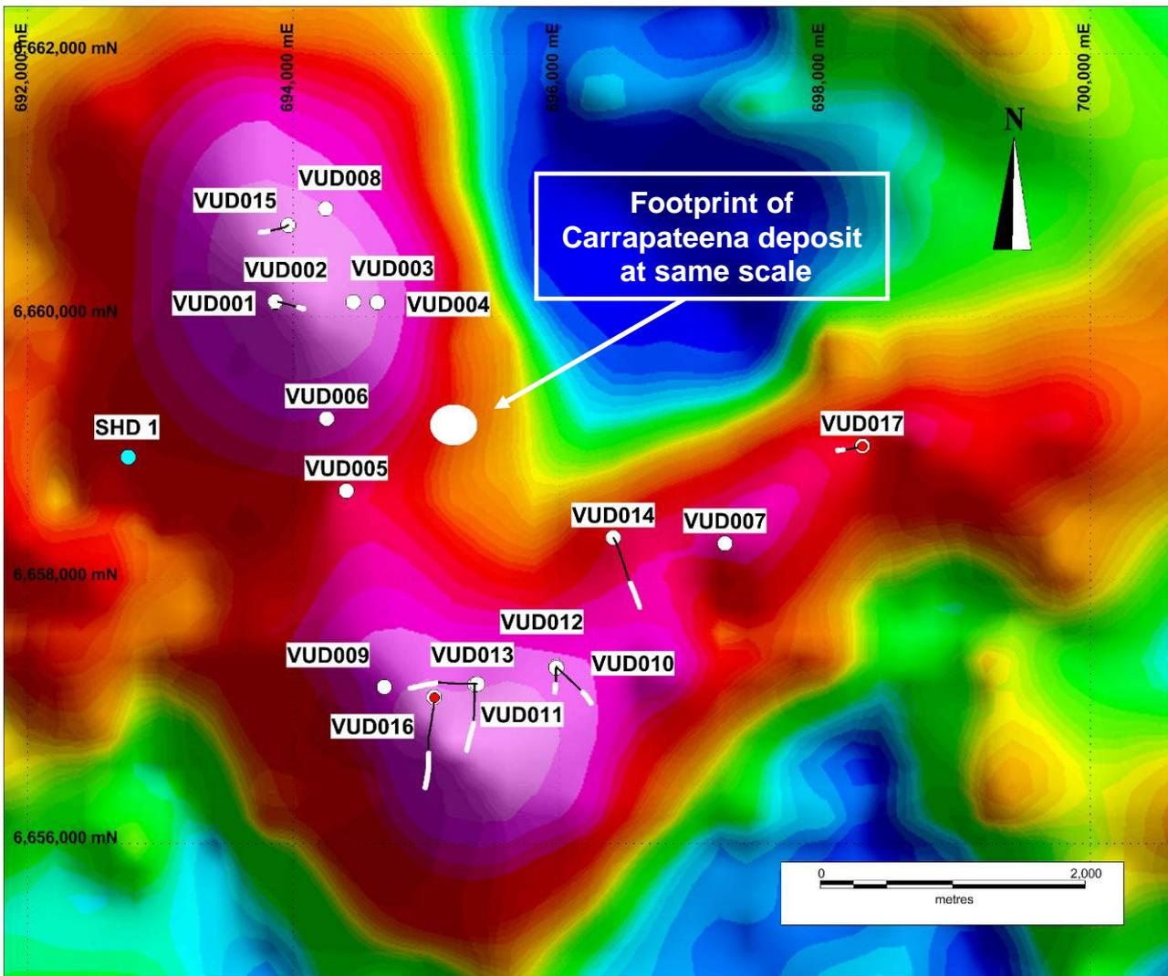
**Figure 1. Residual gravity image of the Vulcan IOCGU Project, showing the location of drill holes completed to date. The surface projection of angled holes are shown as linear traces, with the basement intersection in each shown in white. Also shown at the same scale (as a superimposed white ellipse) is the area occupied by the Carrapateena IOCGU deposit (located approximately 120km to the south southeast). (Datum GDA 94; MGA Zone 53).**
