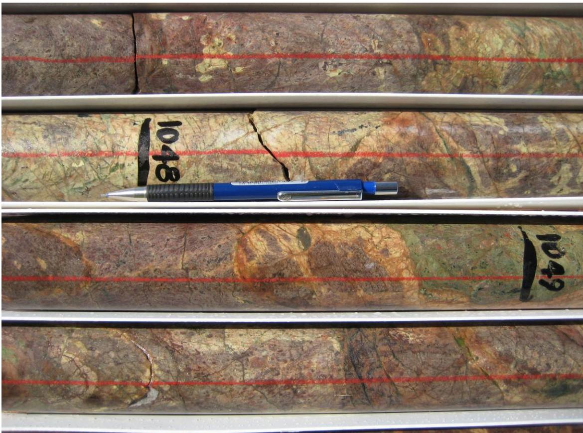
**Figure 3: VUD 16: Strongly sericite altered host rocks; sericite is cream and pale greenish (NQ drill core).**
