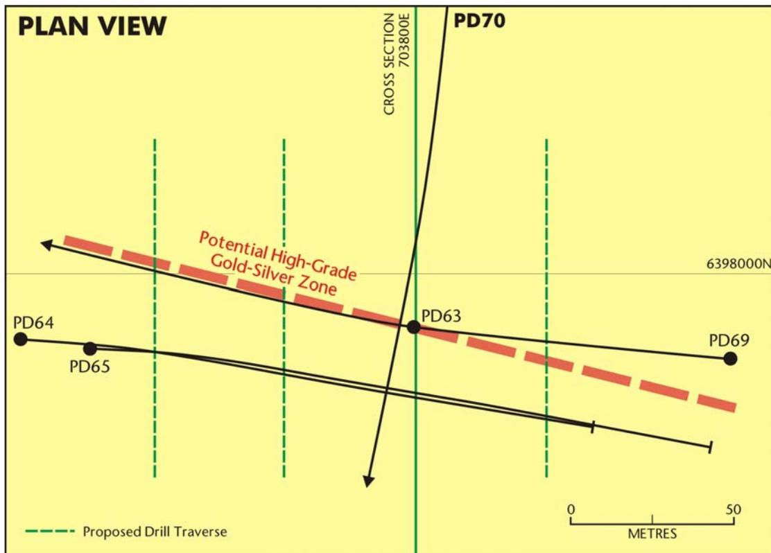
**Figure 1: Parkinson Dam: Drilling plan showing the collar locations and paths (in plan) of recent drill holes, including PD 63, which is essentially vertical in orientation. The interpreted high grade gold-silver target structure at approximately 40m above sea level is shown in red, and is believed to be dipping steeply towards the north. Drilling planned to commence in January 2008 will be conducted on traverses indicated in green. (Datum is AGD 84; AMG Zone 53).**
