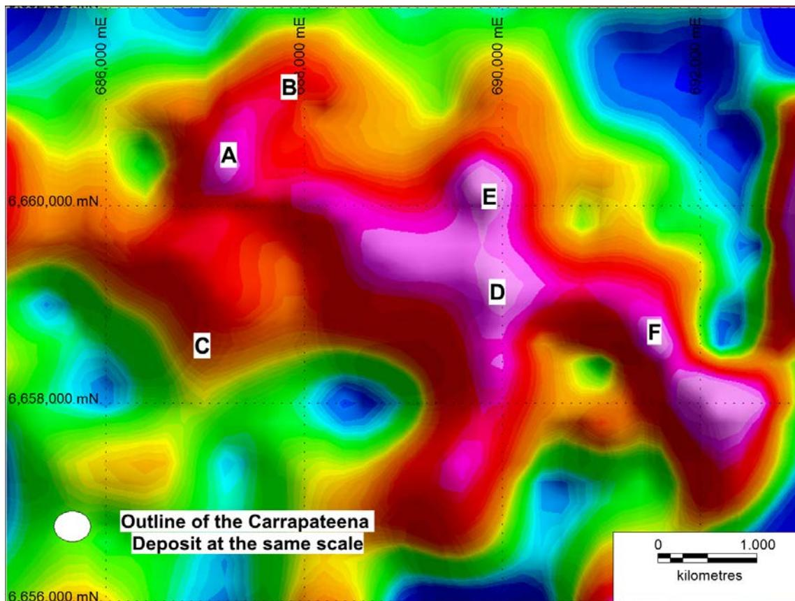
Figure 4. Detailed plan of residual gravity at Vulcan West, based on all available data. Red/magenta colours are areas of stronger residual gravity, generally indicating areas likely to be underlain by denser, more iron-rich rock, potentially IOCG systems. The letter A, B C etc. refer to individual modelled bodies.
